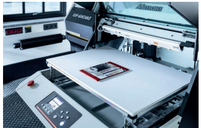
Individual inscription of colored panels is possible with the digital flat bed printing technology © Rowa Group
