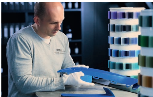
The customer's sample is inspected visually in the Color Competence Center, and the feasibility of the requirements investigated © Rowa Group
