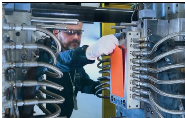
The colorist responsible for color development evaluates the color by means of injection molded sample platelets © Rowa Group
